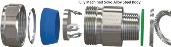
Steel Compression Ring and Santoprene Grommet Unique Precise Grounding Ring Grabs and Retains With Strength Armored Cord Furnished with Sealing Washer and Our HDI Locknut
