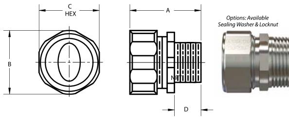
For Securing and Sealing Service Entrance and UF, SE, SEU Cables Entering an Enclosure or Conduit Hub
