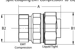
Converts Flexible LT conduit to EMT Conduit Outdoor and Indoor Use with flexible metallic LT conduit or type B flexible non-metallic LT conduit.
